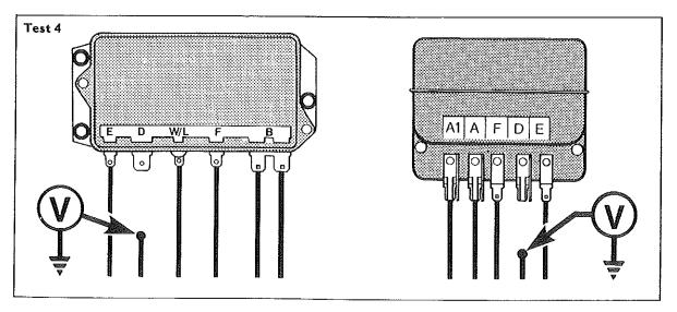
TEST 4: Voltage at 'D' of Control Box
